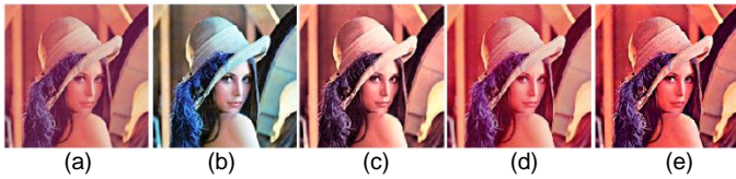
Fig. 1. (a) The color image, (b) the component-wise HE, (c) the image after HE in the HSI model, (d) HE by the average histogram, and (e) the 0.88-rooting by the 2-D QDFT.
